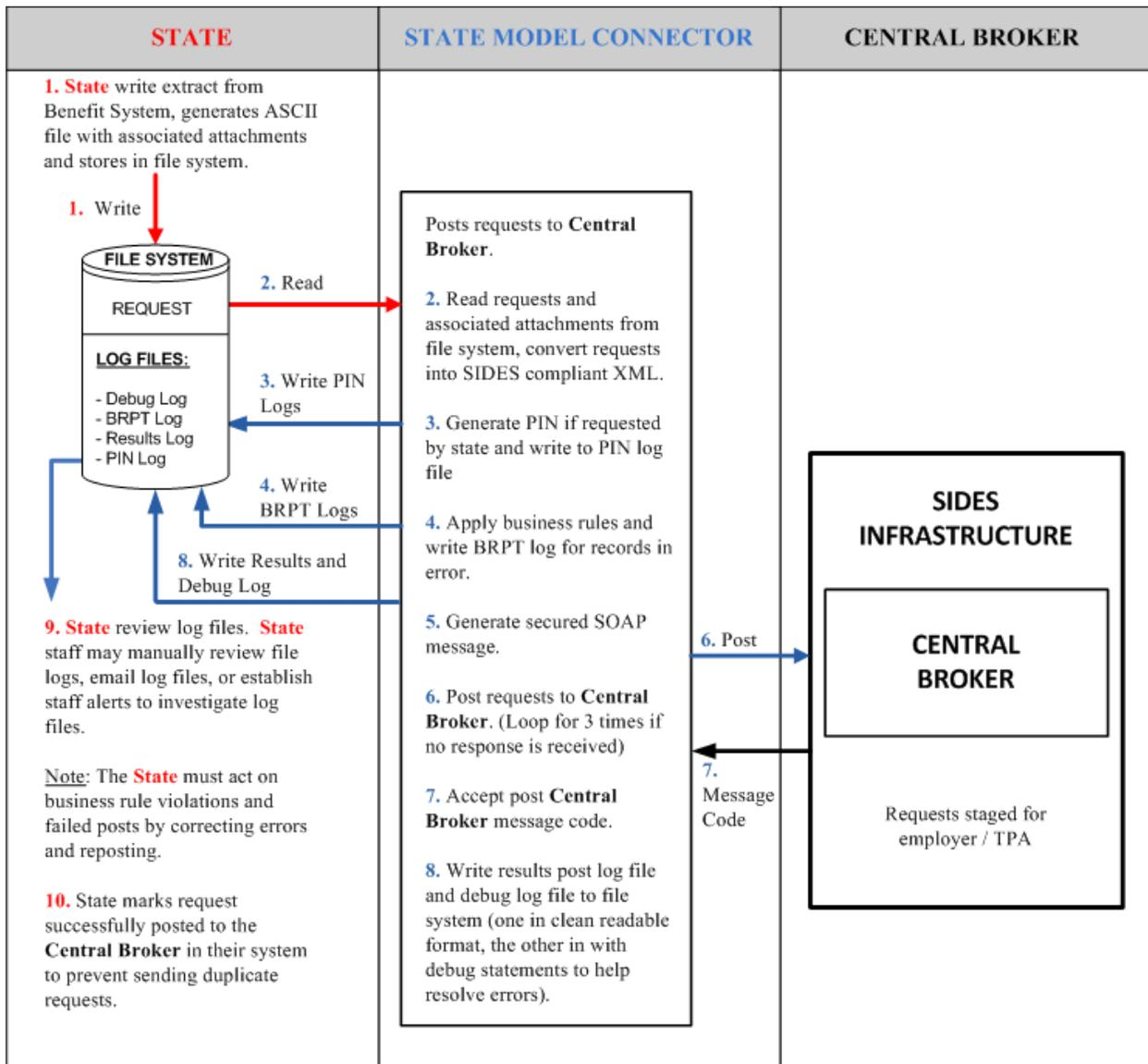
Figure 1. Model Connector Post for ASCII Files
